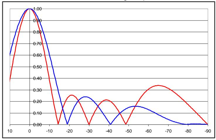
The short spaced pattern looks great and will produce excellent coverage. This elevation pattern also has a bonus – much lower RFR at high depression angles. You can place this antenna lower on a tower and stay under radiation limits. When the time comes to plan your FM repack move, give us a call. We can quickly run the numbers and come up with a economical solution that works well.
