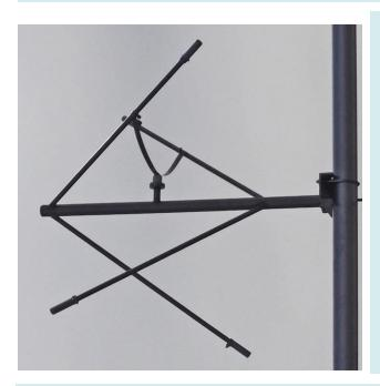
So, how does the TLV antenna solve the problems that this translator has? With the TLV you can stack antennas one on top of another. For the channel 5 antenna, a three or four bay antenna can be mounted further up the tower. Then the channel 4 antenna can be mounted directly below. When spaced properly there is very good electrical isolation between them. Each antenna is fed independently.
